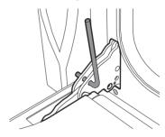
2. Grasp the door on both sides with both hands, lift it forming an angle of around 30° and remove it
