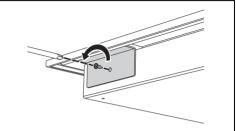
Unscrew the fixing screws and remove the plates for each burner.
