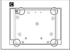
Screw the mounting brackets into the holes shown to fasten the hob correctly to the built-in structure.
