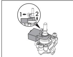
Using a 7 mm wrench, remove the nozzle and replace it with one suitable for the new type of gas, following the instructions in the relative tables (see "Types of gas and countries").
