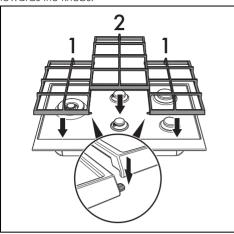
Insert the central pan support (2) by slotting the recesses onto the lugs of the lateral pan supports.
